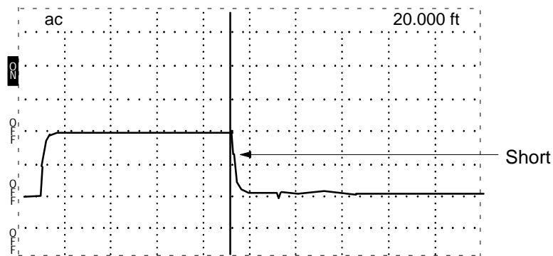
Figure 1-9: Short in the Cable
